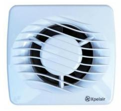
The DX100 is IP55 rated and suitable for 220V-240V 50Hz mains operation. Class B insulation for operation in ambient temperatures up to 40°C and are fitted with a thermal cut out.
